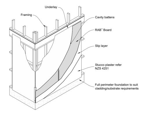
RAB<sup>™</sup> Board used as backing board for stucco plaster/proprietary cladding systems
